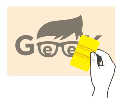
1 Lay dacal Face up on a smooth hard surface. Squeegee the surface to ensure good contact between the pre-mask and the vinyl beneath it.
