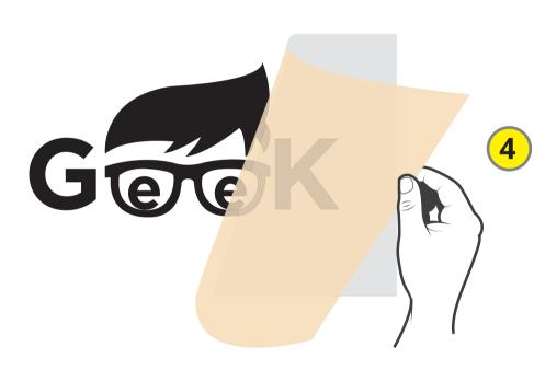
To expose product, pull pre-masking away using a continuous motion. If bubbles occur in the letters, simply prick with a needle and smooth. Do not use a knife or razor.
