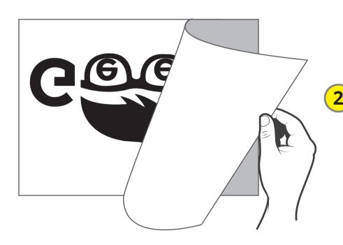
Lay dacal flat Face down. Slowly remove backing paper from the pre-mask. Pulling straight back and flat as shown.
